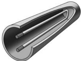
FIG. N - Pipe wells
